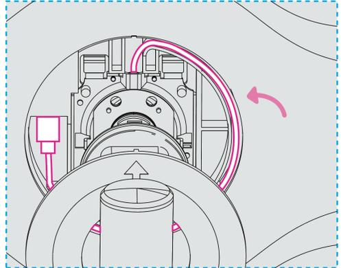
Cross the cable over the top and insert it into the power interface at the back of the display.
