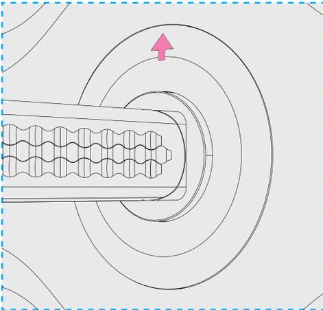
Align the two indicator marks and position to fasten the monitor cover to the Monitor.
